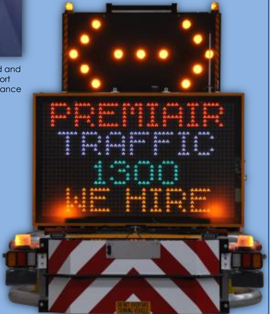
Full Colour Type-B Variable Message Board (320mm Font)
