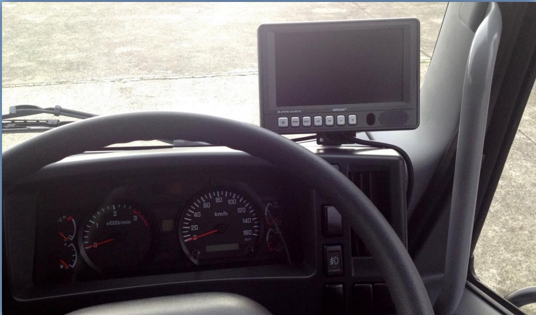
Multi-view, split screen video monitor enables operator to safely stay in cabin with the ability to monitor surroundings at all times
